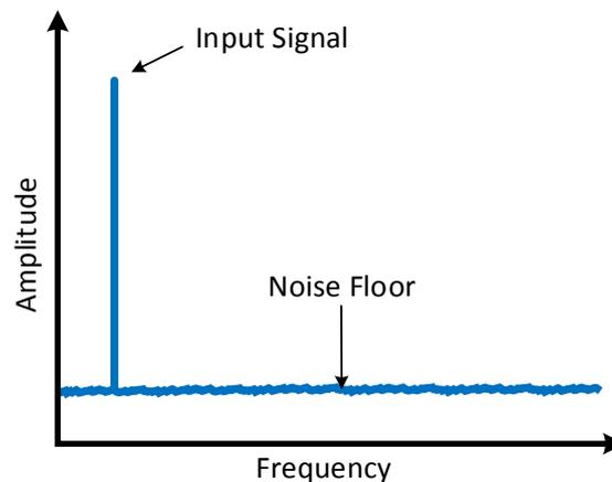
Noise exists in digital systems too, but the noise sources and coupling mechanisms are different to those found in analog systems. The transistors used in digital circuits all generate noise (they are fundamentally analog components after all), but the level of noise they generate is well below that required to cause the digital signal to change state (e.g. flip from a '1' to a '0'). A digital signal does not therefore accumulate noise just by passing through a digital circuit.
