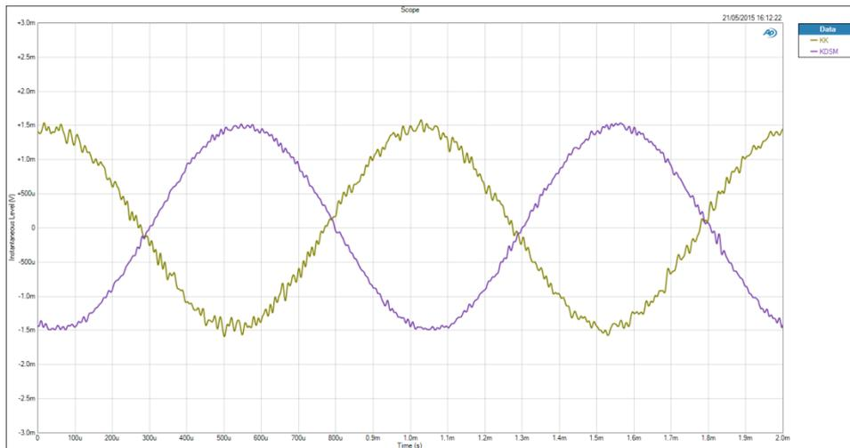
Even at this low volume setting the purple DSM output appears to be a faithful analog representation of the input signal, with no sign of any ‘digital’ artefacts. The DSM also appears to add less noise to the signal than the Kontrol. This is confirmed by looking at the same signals in the frequency domain.
