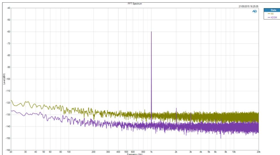
The purple noise floor of the DSM is some 8dB lower than the Kontrol across the audio band.
