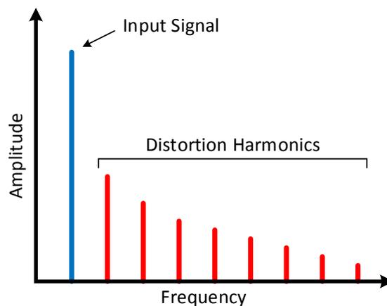
All active analog components (e.g. diodes, transistors, op-amps, etc.) and some passive ones (e.g. transformers, capacitors, inductors) will generate distortion to some degree. In an analog pre-amp, the primary sources of distortion are usually the switching transistors used for source selection and attenuation (volume stepping).
