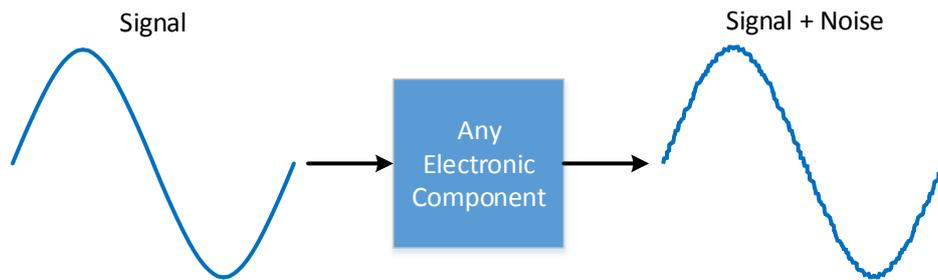
The level of noise can be measured either by looking directly at the signal in the time-domain (as above), or alternatively, by observing the noise 'floor' in the frequency domain.
