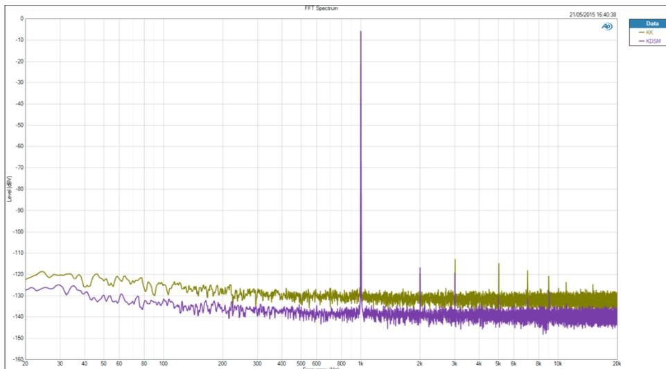
Distortion levels at the 2<sup>nd</sup> harmonic frequency (2kHz) are roughly equal between the two products, but the Klimax generates higher levels of all the higher order products. High order distortion is generally considered to be more objectionable than low order distortion.
