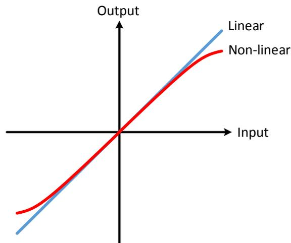
A non-linear transfer function distorts the original signal by generating new signals at multiples of the input frequency. These new signals are called harmonics, hence the term 'harmonic distortion'. Harmonic distortion is easily identified by the presence of unwanted frequencies in the output spectrum.
