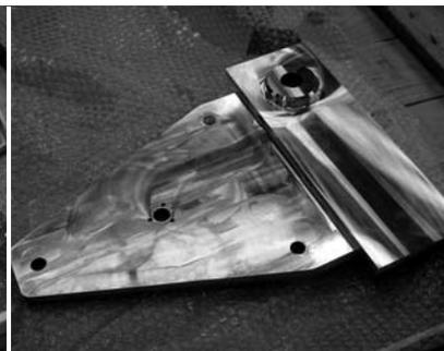
■ The Keel is diamond machined for the smoothest finish possible
